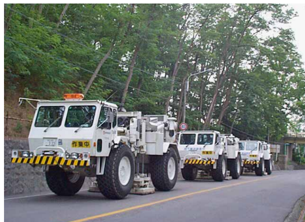
△ Land seismic survey using a vibroseis vehicles
