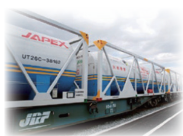
Transportation of LNG by railway tank containers
