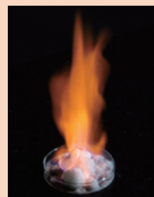
Artificial methane hydrate set alight
