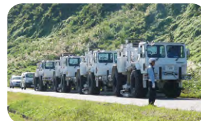
Vibrator trucks at work
